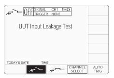
The above default screen has auto-selected the open-circuit output, as indicated by the icon in the top left corner, and the highlighted screen key on the bottom row.
