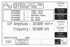
Both channel key labels and the Dual channel label are highlighted, and the legend in the box at the top of the screen shows the two channels selected, the Master written first.
