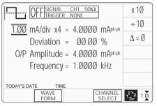
The above default screen has auto-selected the symmetrical square waveform, as indicated by the icon in the top left corner. Frequency is variable between 10.000Hz and 100.00kHz. Frequency has defaulted to 1kHz, deviation  $\Delta$  to zero, and output current to 4.0000mAp-p. The Duty Cycle is fixed at a nominal 50%.
