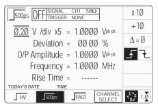
The above default screen has auto-selected a frequency of 1MHz, a rise time of 500ps, zero deviation and an output level of 1Vpk-pk.
