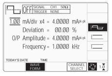
Both polarities of DC Current output are listed merely as different waveforms. As an example, pressing the \_\_\_\_\_ key from the setup shown above will present the DC function screen, showing negative values selected (of course, the frequency parameter has disappeared from the screen):
