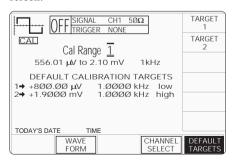
When you select target 2 by pressing its soft key, the Target Amplitude and Frequency will be displayed below the current Output Amplitude as shown in the following **Adjustment** screen illustration:
