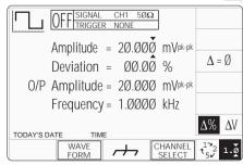
Fig. 4.4.2 Typical Screen in Direct Mode
