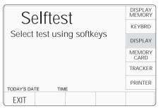
Selecting 'DISPLAY' transfers to the 'Display test.' screen. This invites a user to use the front panel 'tab' () key to move the dark band down the screen, up to the top, and down again, thus testing all the display elements on the screen:
