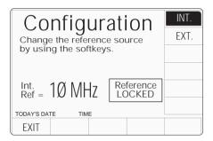
When switched to 'EXT.', use the up/down cursor control or spinwheel to inform the 9500B of the source frequency. Ensure that the required source is connected and operating.
