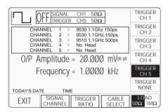
This channel must be allocated as a 'cable' channel; accessed by pressing the 'CABLE SELECT' key. A new screen is presented:
