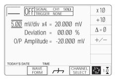
Once into DC function, it is not necessary to change the waveform to change polarity. Pressing the +/- screen key toggles between positive and negative DC Voltage. The polarity selection is shown by the function icon in the top left corner, confirmed by the + or - sign on the O/P Amplitude value.
