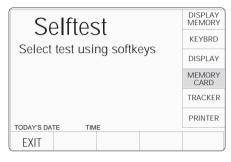
Pressing the MEMORY CARD key on the 'Select test' menu screen transfers to the 'Card slot test.' screen. This invites a user to select the memory card slot to be tested, and presents an 'Overwrite' warning:
