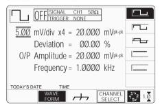
The WAVEFORM key label is highlighted to indicate that waveform selection is available, as is the presently-selected waveform icon.
