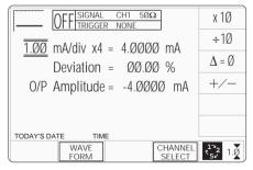
Once into DC function, it is not necessary to change the waveform to change polarity. Pressing the +/- screen key toggles between positive and negative DC Current. The polarity selection is shown by the function icon in the top left corner, confirmed by the + or - sign on the O/P Amplitude value.
