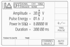
The above default screen has auto-selected the positive pulse waveform, as indicated by the icon in the top left corner. Amplitude is variable between 5 Volts and 20 Volts (default). Pulse Energy is variable between 1.6 Joules (default) and 50 Joules. Power into  $50\Omega$  and Pulse Duration are calculated from the voltage and energy settings.
