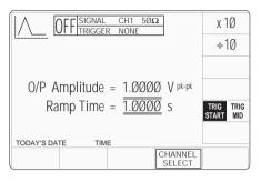
The 9500B has auto-selected a Ramp Time of 1.0000s. Trigger is auto-selected: 'TRIG START', not 'TRIG MID'. O/P Amplitude is fixed at 1.0000V.
