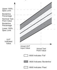
When in Procedure mode, the direct-printing certificate (Style 1), and the data on the 'Results' card, will report 'Borderline' test results. Users have access via Configuration mode to set the percentage for borderline reporting.
