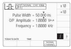
The above default screen has selected a 50ns Pulse Width at a frequency of 1MHz.. Output amplitude is fixed at 1Vpk-pk into 500hm.
