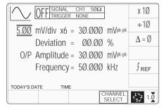
The above default screen has auto-selected the frequency of 50kHz. Deviation has defaulted to zero, and output voltage to 30.000mVp-p. Frequency is variable between 0.1Hz and 1.1GHz (variant 9500B/1100 — for other variants refer to specifications in *Section 7*).
