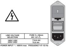
A window in the fuse drawer allows the line voltage selection to be inspected. To inspect the fuse rating the fuse drawer must be taken out (Refer to sub-section 2.7.4. First switch off and remove the power cable).
