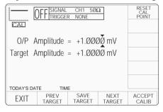
This screen initially shows the value to which the 9500B output is presently set, and the value of the selected target amplitude (whether 'default' or 'saved'). Note that on these values, triangular cursors indicate which digit will change when using the cursor keys or spinwheel. When transferring, using the 'tab' key, the cursor always moves to the least significant digit on the other value.
