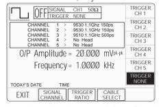
been allocated to triggers. This is confirmed by the legend in the top central box and the right side screen keys.
