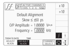
The above default screen has auto-selected Default Alignment', as indicated by the top line of text and the highlighted screen key on the bottom row. The unequallized (default) alignment has a maximum skew of  $\pm 50 ps$  between channels. The amplitude and default frequency are also shown on the screen.
