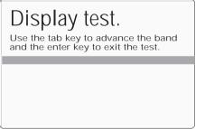
The screen text will shift automatically so as not to obscure the band as it jumps back to the top of the screen. If there are elements of the screen which do not show light in the light background or dark in the dark band as it is advanced down the screen, then this implies a failure. Rectification will require access to the internal circuitry, so no further user action is recommended, except to report the result to your Fluke Service Center.
