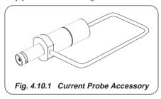
With the 9500B 'Auxiliary' Current function selected and output on, the output current in the loop can be set to the UUT oscilloscope's current probe calibration points, using 9500B front panel controls.
