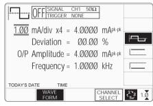
The WAVEFORM key label is highlighted to indicate that waveform selection is available, as is the presently-selected waveform icon.
