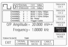
Note that the expected load key in the bottom right corner is now de-activated, and the trigger state legend in the top central box is fixed on  $50\Omega$ . A further selection is available, to choose the trigger ratio.
